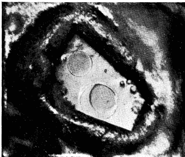
Figure 3 Two SiC tunnel diodes on the same p+ SiC chip. The two circular regions are slightly depressed areas wet by the Si dots; that on the left has a diameter of 0.014 inch. The peripheral ridge is a tungsten, silicon, and carbon residue produced when the SiC melted into a tungsten tab during violent heat treatment at 2200°C.
