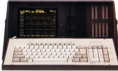
PM 3655 100 MHz Logic Analyzer (up to 96 channels)
