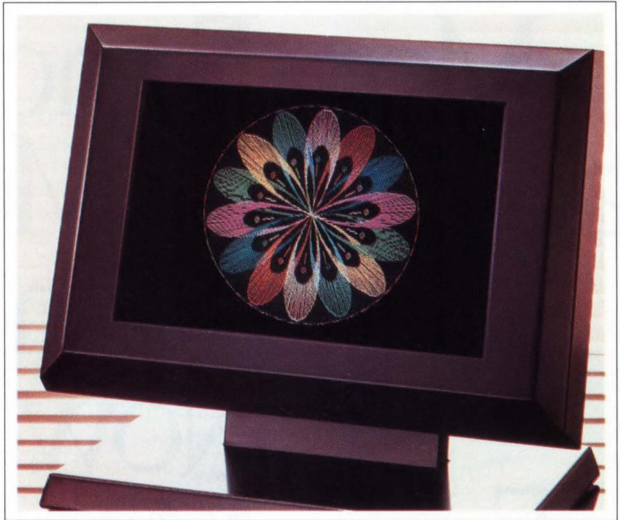
*Active-matrix TFT technology enables this LCD panel to reproduce eight colors that have high contrast and  $640 \times (200 \times 3)$  pixels of resolution.*
