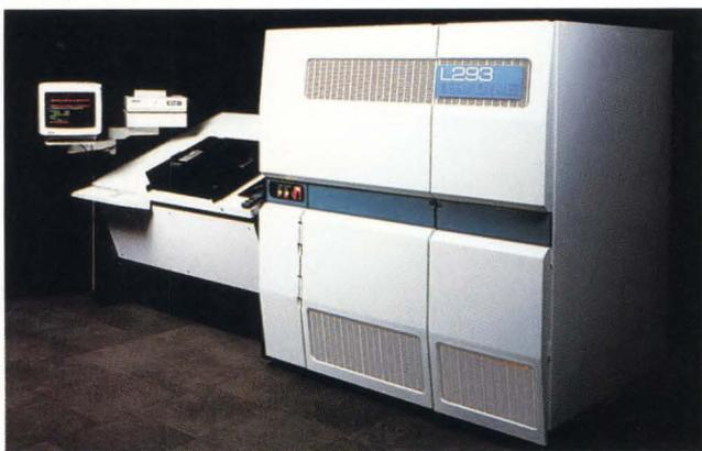
The L293 VLSI Module Test System.
