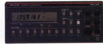
PM2535 6½ digit System Multimeter with 0.0025% basic dc accuracy, up to 100 readings per second, IEEE-488.
