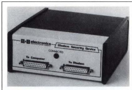
a hacker steals a user's password, the password is unusable because the thief will not be at the user's phone number. The unit features a 50-number directory of password/phone number combinations, EEPROM storage for power-failure protection, and a systems manager that can disable the call-back procedure as an alternative. \$129.95.
