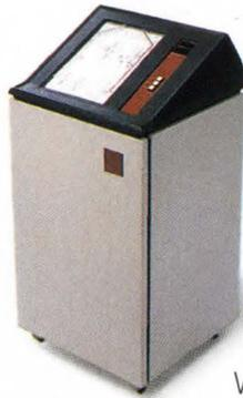
Versatec responded with a whole new line of wide carriage plotters. In widths from 20 to a whopping 72 inches. Plus the ability to print on paper or vellum in clear or matte finishes. A little later we'd add 200 ppi resolution, the first RS-232 and direct CRT interfaces, first I/O multiplexer, minicomputer graphics software, universal graphics software and a few dozen other innovations.
