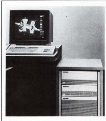
ers. In addition, it contains 4M bytes of RAM expandable to 16M bytes, a 16-in. color monitor with 1280x1024-pixel resolution, and the company's SRX graphics subsystem, which can be expanded from 8 to 32 color planes. The system is compatible with a range of 3D mechanical CAE and CAD software available from McDonnell
