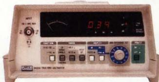
8920A 3½ digit Wideband True RMS AC Multimeter with autoranging, dB and rear panel linear analog output.
