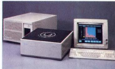
Thanks to its high degree of integration, the LV 500 rarely needs calibration. DUT fixturing is simplified. And capacitance loading is reduced to about 25 pF, further contributing to the system's accurate results. And it is compatible with virtually all logic simulators.
