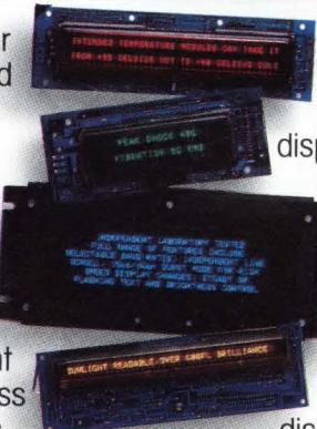
XT and XTB features include selectable baud rates, 15 microsecond-per-character burst mode for high-speed display changes, steady or flashing characters, and brightness control.
