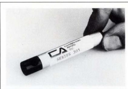
a factory preset limit. Operating over a 5 to 70°C range, the switch features a self-heated glass-bead thermister, which compensates for ambient temperature, air speed, altitude, and relative humidity, and can sense a reversal in air flow. The switch is cooled by the same air stream that cools the host equipment, and measures 3 x 0.5 in. From \$15.
