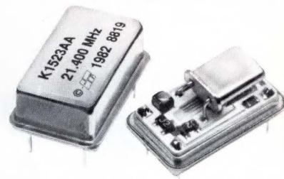
The K1523AA Voltage Controlled Crystal Oscillator allows system designer to phase lock to a reference standard. For LANs, computer shared management systems, communications, A/D interface. 3 MHz to 35 MHz,  $\pm 50$  ppm per volt sensitivity.  $\pm 25$  ppm stability. TTL or CMOS compatible.
