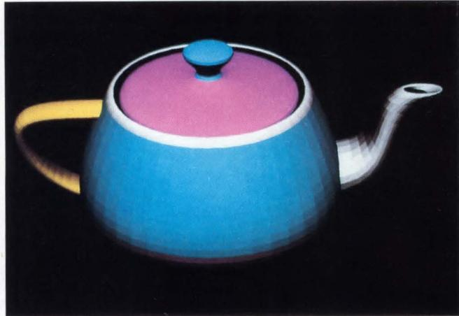
**Fig 2—**When no shading algorithms are applied to this graphical rendering of a teapot, each polygon has only one color assigned to it, so the teapot appears to have a nonsmooth surface.
