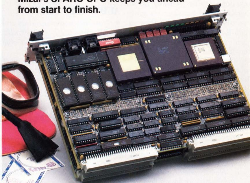
You'll be favored to win with Mizar's MZ 7170, the VME processor with triple crown features. With the power of SPARC™ and the speed of zero wait-state SRAM, the MZ 7170 lets you run your application in record time. All for a price that keeps you on track.
