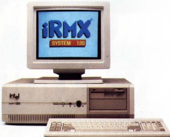
*System 120. The first integrated real-time system based on the AT-bus with iRMX® software.*
