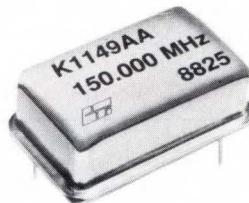
MECL 10KH-based design for improved rise and fall times, duty cycle, noise margin, and power supply rejection. Open emitter output for user selection of load. Complementary outputs available, various pinouts also available.
