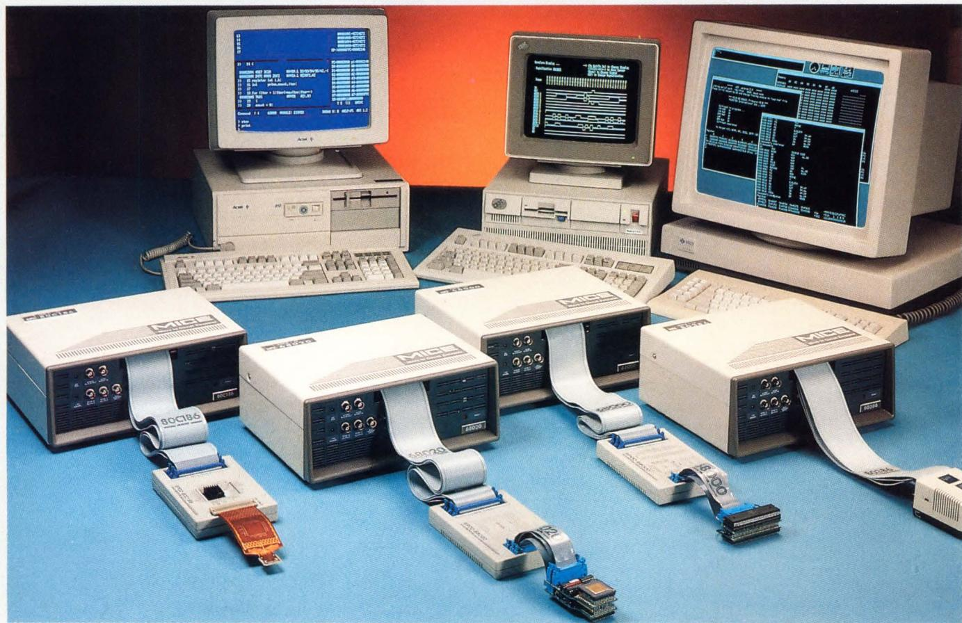
**M**ICROTEK offers a complete line of MICE (Micro-In-Circuit Emulator) for most popular 8, 16 and 32-bit microprocessors. These series of MICE are capable of debugging high speed targets without accumulating wait state, e.g. 25 MHz for 68020, 16 MHz for 68000/80C186. Protected Mode in 80386, coprocessor emulation in 16/32 bit series and bus/execution breakpoints in all series, are few examples of MICE powerful emulation features designed to meet advanced development needs.
