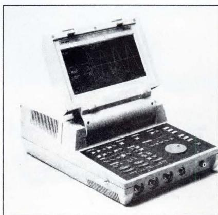
In addition to displaying waveforms, the oscilloscope allows you to make a variety of waveform measurements. These include time between reference points, voltage differences, p-p and rms voltages,
