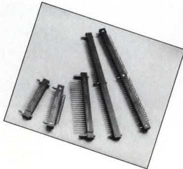
**KA Series—Sub-Miniature LIF/PCB Connectors** • The choice in demanding military and industrial applications • 17-320 position models with average contact insertion force of 1 ounce • Removable p.c., wire wrap, solder and crimp terminals • Integral guide and locking hardware.
