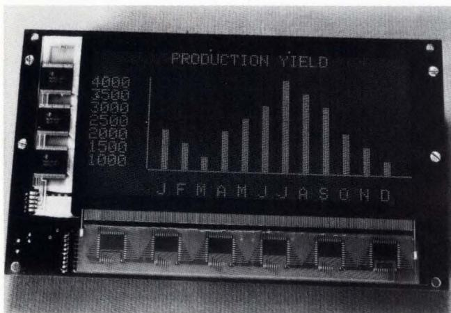
**Dot-matrix plasma displays are useful for charting graphic data.** This 192-column by 88-row panel from Dale Electronics is used in computer terminals and other systems that require self-contained readouts.
