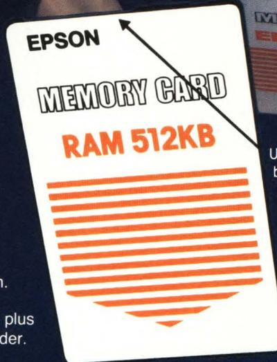
User replaceable battery for SRAM cards . . . plus write protect switch.
