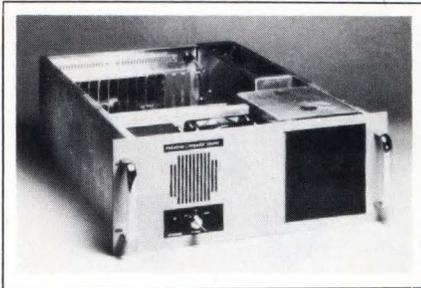
the chassis delivers full PC/AT functionality. The rugged steel enclosure includes a disk-carrier assembly that can hold as many as four half-height drives, a drive-area cover door, a system reset button, and a 200W power supply with a filtered cooling system. A positive-pressure buildup inside the chassis prevents dust particles from damaging any installed drives. From \$1395.
