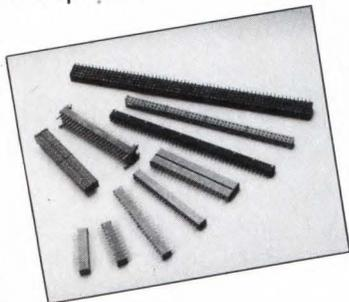
**KG Series—Sub-Miniature Low Profile LIF/PCB Connectors** • .100 x .100 grid from 22-90 positions • .240 height between parallel boards, sandwich style • Mother/daughter board, board to chassis and other applications • Inductance as low as 50% of comparable designs.
