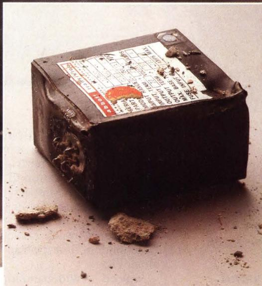
In a Navy test, a Tomahawk cruise missile exploded into a concrete building. When the dust settled, little remained but gravel and fragments of casing.
