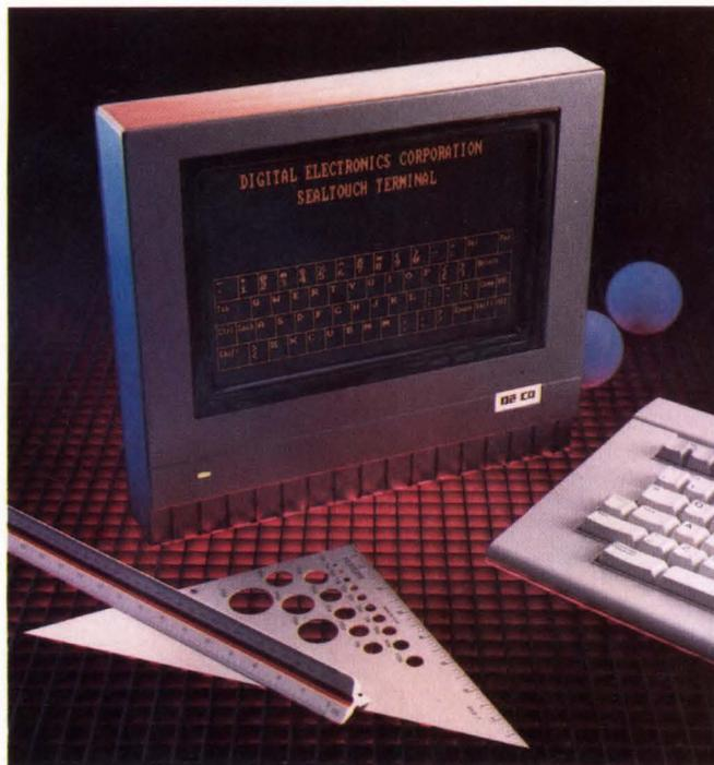
With its characteristic yellow-on-black color, EL displays provide high contrast. This electroluminescent flat-panel display from Digital Electronics Corp has an infrared touchscreen and is completely sealed in a cast aluminum case for use in harsh environments.
