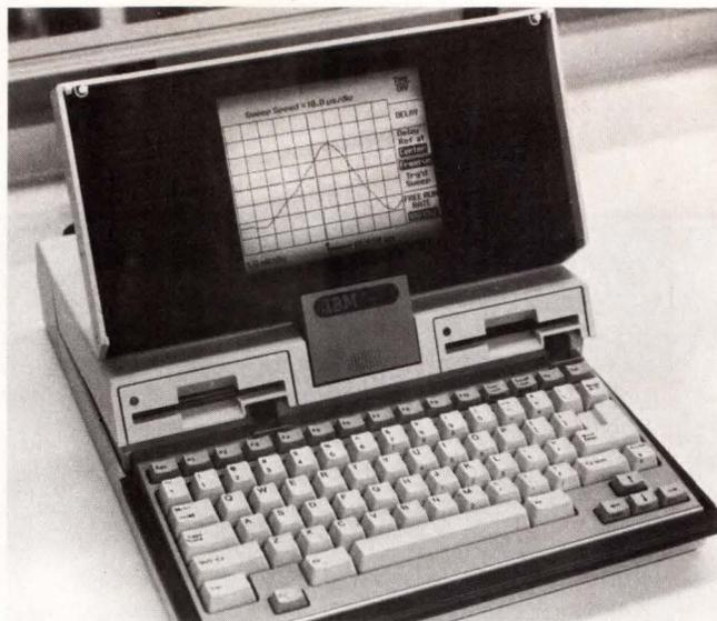
*An IBM PC portable demonstrates the use of Alphasil's active-matrix LCD. The portable system provides a way for OEMs to demonstrate their own applications before investing in a custom or semicustom display.*
