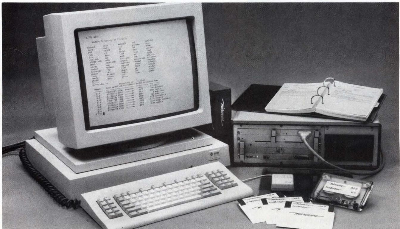
*Unix systems can host real-time software development efforts with the Unibridge software package. The software links target systems based on the OS-9 real-time operating system to Unix-based hosts via Ethernet and TCP/IP.*
