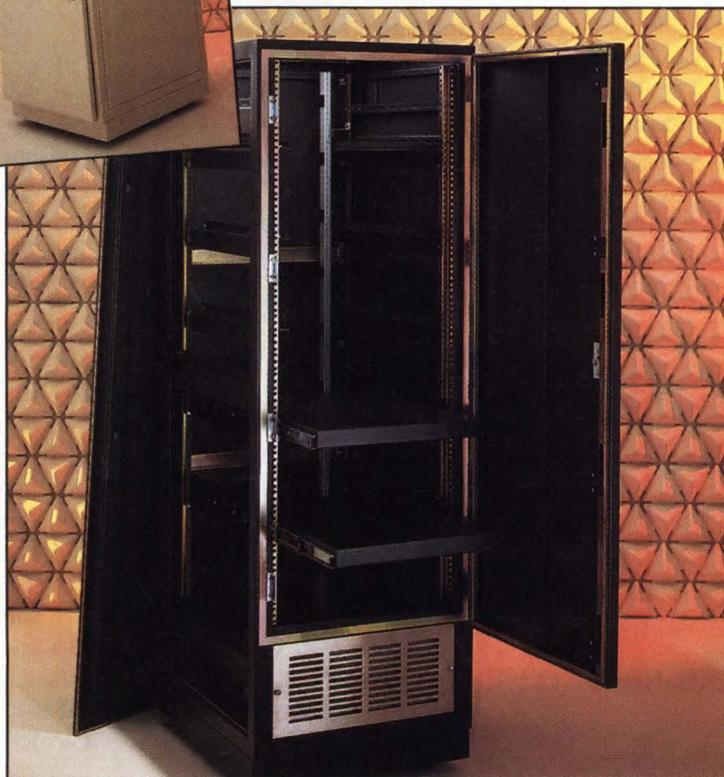
Emcor offers a choice of shielding solutions, all of which are tested to MIL STD 285. These enclosures combine high strength with modular options and attractive esthetics. Emcor's commercial EMI/RFI enclosures are fabricated from 14-gauge cold-rolled steel and are fully zinc-plated. Our Tempest-style enclosures provide even higher levels of attenuation. They are fabricated from 12-gauge cold-rolled steel, nickel-plated and feature a unique latching system and door design (patent pending).
