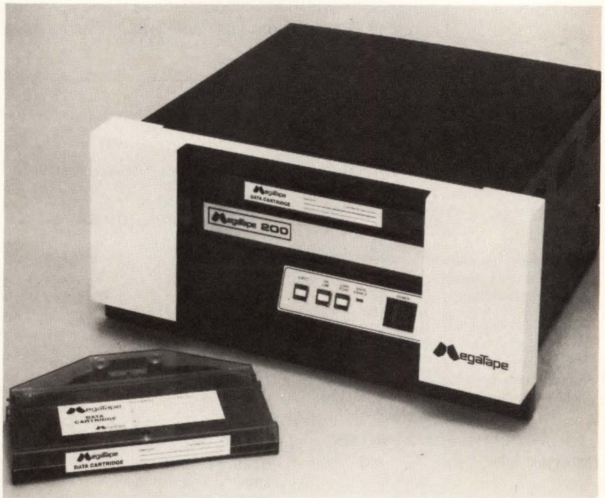
Figure 1: Megatape 1/2" streaming drive and cartridge. Cartridge holds 1000 ft.
