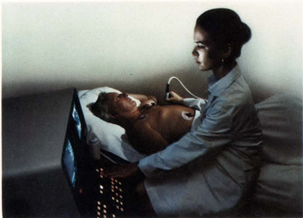
Figure 5: GE's PASS (Phased Array Scanning System for Echocardiography) has two separate monitors displaying menu selections and the 2-D image.
