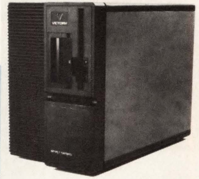
Figure 1: The Victory SPIRIT series computers are Intel iAPX 186 (80186)-based systems supporting the CP/M-86, MP/M-86 and CP/M-80 operating systems
