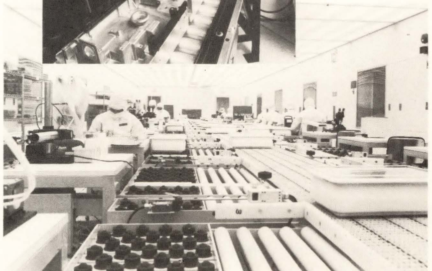
Figure 2: Interior of Class 100 clean tunnel. Tunnel allows progressive manufacturing within controlled environment required by Winchesters.
