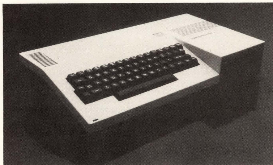
Figure 2: STM Electronics' Pied Piper I includes 64 Kbytes of RAM, full ASCII keyboard, high capacity minifloppy with 256 Kbytes of storage, and built-in printer interface for Centronics/Epson-type devices.
