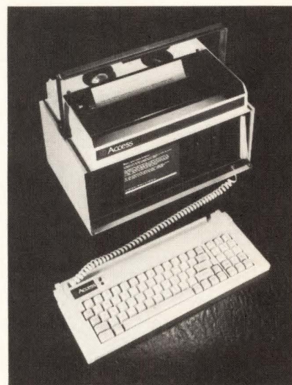
Figure 3: Access portable computer with integrated printer, acoustic modem and a 9" CRT display.
