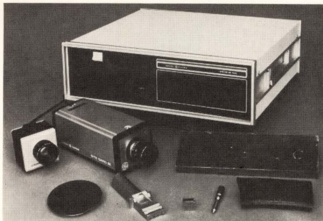
Figure 3: GE IPARS Vision system reads characters on various surfaces.
