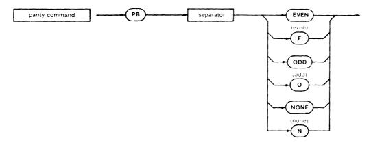
The parity command defines a parity bit to be generated and checked for the selected port. Parity is an error detection scheme that uses an extra bit appended after the last data bit of each word. This bit is set so that the total number of 1-bits in each word is always even or odd.
