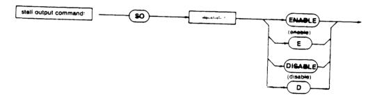
The stall output command defines the state of the stall output feature.
