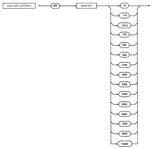
The baud rate command changes the baud rate of the selected port to that specified by the command argument. Baud rate is the bit transfer rate in bits per second, including start, stop, parity, and unused bits.
