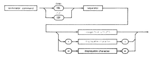
The terminator command defines a character that will be used to identify the end of a line or file. When received with incoming data, a terminator will generate an interrupt if enabled by the user program.
