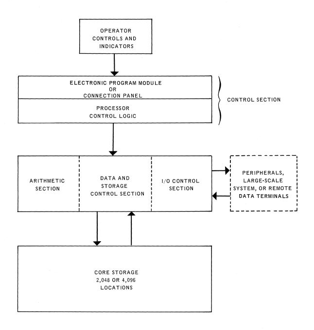
Figure 3-1. UNIVAC 1005 Central Processor - Functional Block Diagram
