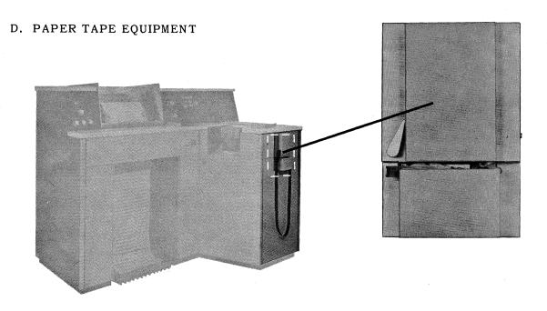
Figure 4-7. Paper Tape Reader - Mounted on Card Reader
