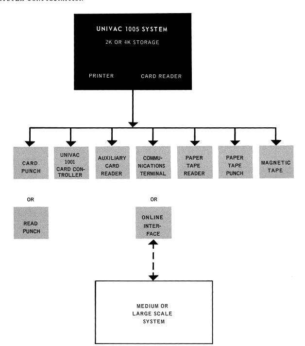
Figure 2-3. Maximum System Configuration
