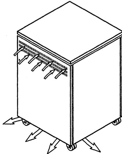
**Figure 4-2. Direction of Airflow through a 3720**
