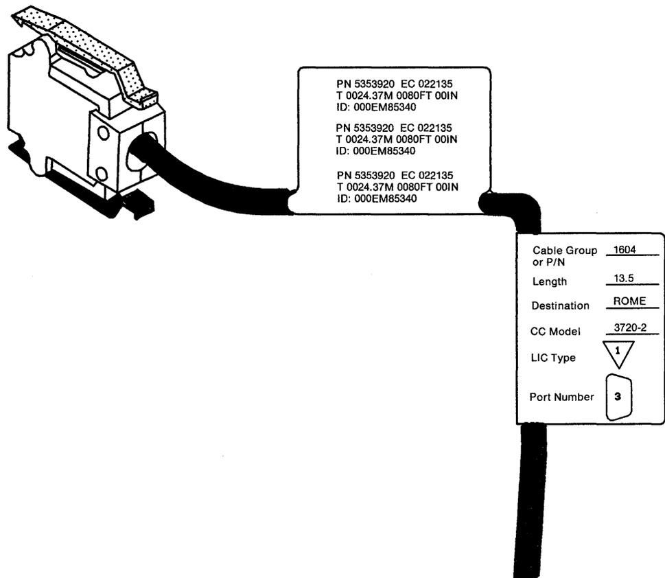
Figure 7-4. Label to be Attached to a LIC Cable
