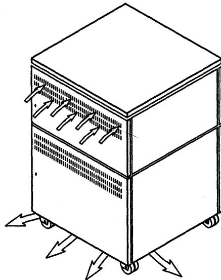
**Figure 4-3. Direction of Airflow through a 3720 with a 3721**
