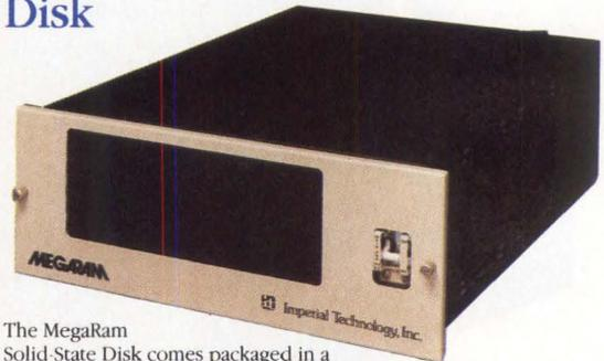
The MegaRam Solid-State Disk comes packaged in a 7-inch high, 19-inch rack mounted chassis with its own controller, power supply and blower assemblies.
