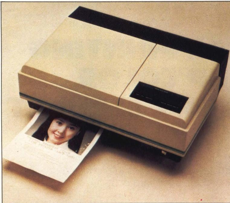
**Producing B-size output,** Panasonic's 400-dpi thermal printer uses a half-tone dither technique to generate 256,000 color shades.
