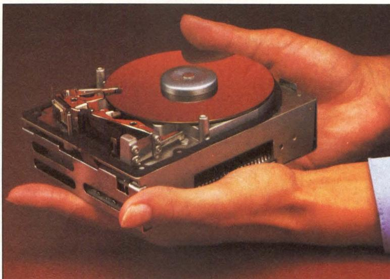
**Micro-Winchesters**, such as Hewlett-Packard's HP97501A, usually employ 3½-inch disks. An exception is SyQuest's line of sub-4-inch fixed and removable drives, which use 3.9-inch media.
