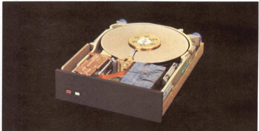
**A voice-coil motor** helps the 50M-byte Microscience HH-1050 achieve an average access time of 35 msec.
