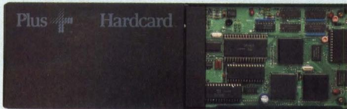
**Measuring 1 by 4 by 13 inches,** Plus Development's Hardcard is a 10M-byte hard disk drive that plugs into a PC expansion slot.
