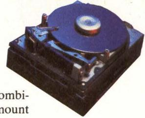
3.9-inch media. The drives measure 1.62 inches by 4.8 inches by 8 inches. Nevertheless, two SyQuest drives will fit in the space occupied by a minifloppy drive. SyQuest, the leading manufacturer of full-size removable-cartridge Winchester, is the only sub-4-inch disk manufacturer to offer removable cartridges.
