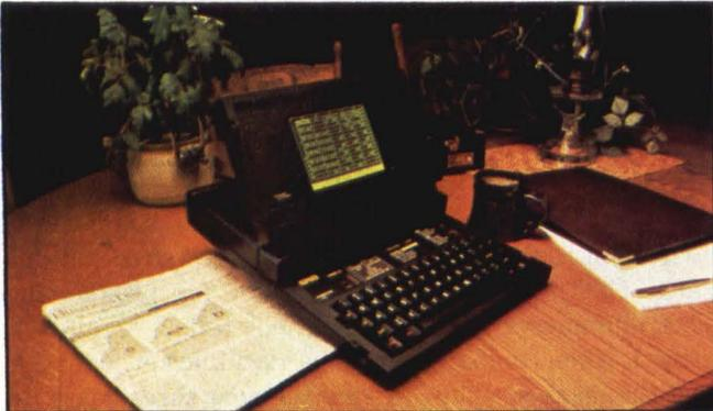
Grid Systems' portable microcomputer incorporates a Sharp electroluminescent display. Emulating DEC VT100 or IBM 3270 systems, the Compass can be used as an intelligent terminal in the office or as a portable computer on the road. The Sharp display provides users with graphics and alphanumeric capability and enables the Compass to fold into a 2- x 11½- x 15-inch package.
