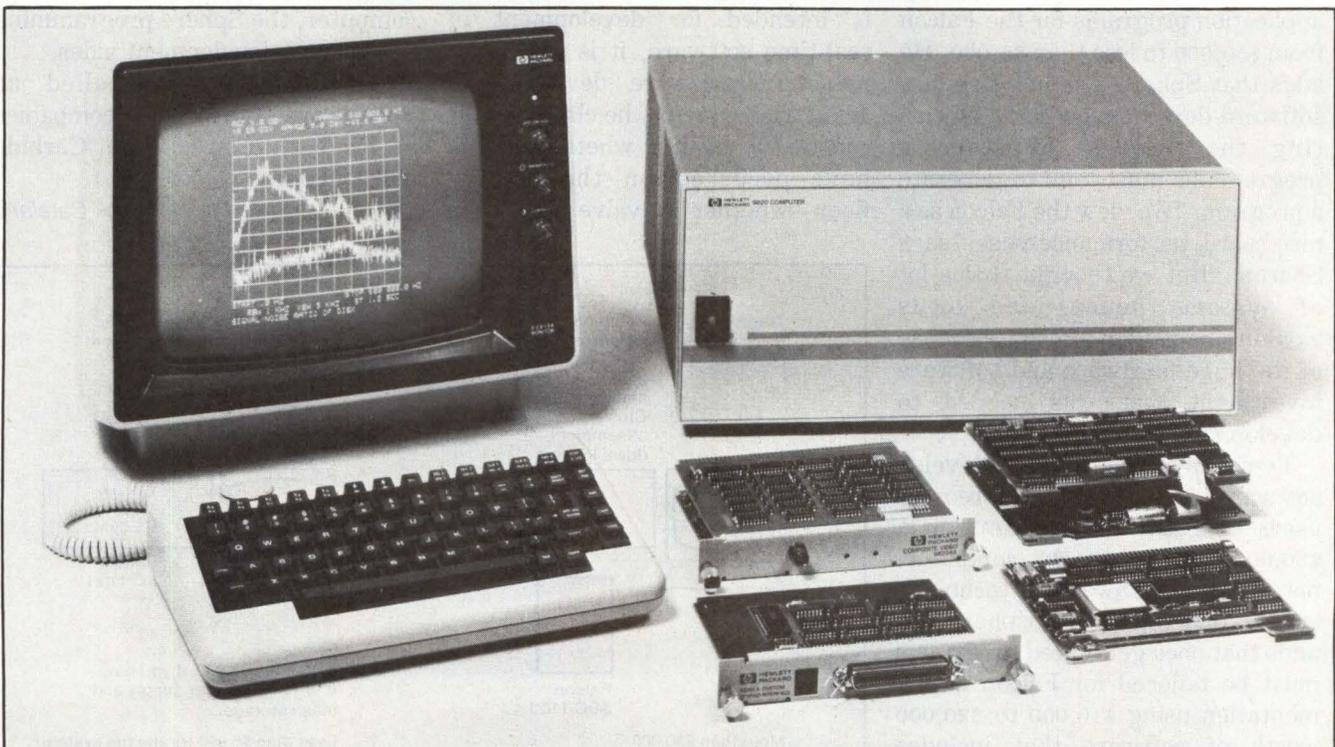
The HP Series 200 model 20 instrument controller is an addition to the company's family of MC68000-based microcomputers. Among the product's specialized features for instrument control are multiple option slots for connecting instruments, an optional bubble-memory card and an EPROM card for use in harsh environments.
