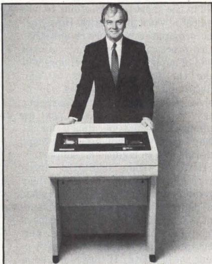
High-quality print was top priority in the design of the Centronics Linewriter 400 band printer. The company expects to garner significant OEM contracts for the printer.
