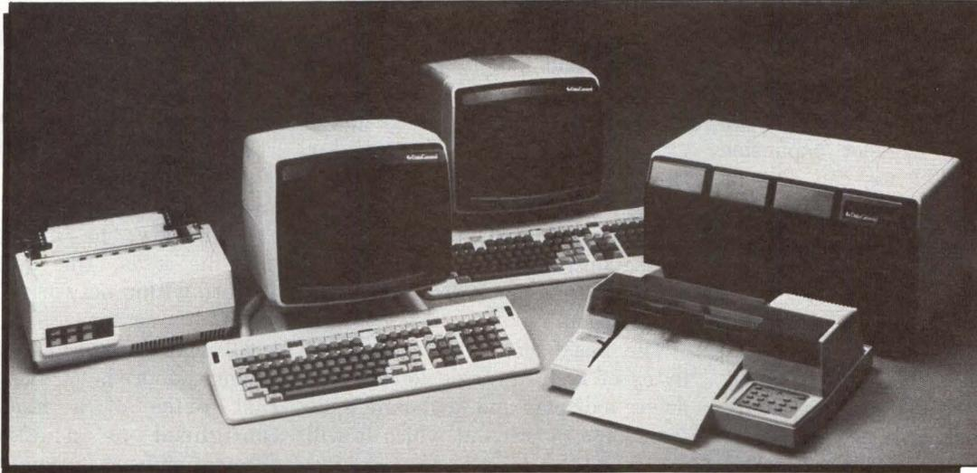
DG's microEclipse-based Desktop Generation is available in a variety of configurations ranging from a \$3,165 single-user system that includes an Intel 8086 co-processor for running MS-DOS and CP/M-86 packages. Multiuser configurations supporting as many as 12 terminals are possible. With the system, DG is introducing a new Mannesmann Tally printer (left) and a Hewlett-Packard plotter.
