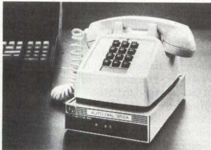
The modem's self-test system and multiple DIP switches permit any user to install and adapt the Auto Dial 212A to virtually any computer or terminal. The Auto Dial 212A also features a low parts count for low cost and high reliability. Three vendor-developed microprocessors compress the entire range of modem functions within 12 ICs, all contained on one PC board. Price is less than \$600 in single-unit quantities. **U.S. Robotics Inc.**, 1123 W. Washington Blvd., Chicago, Ill. 60607.
