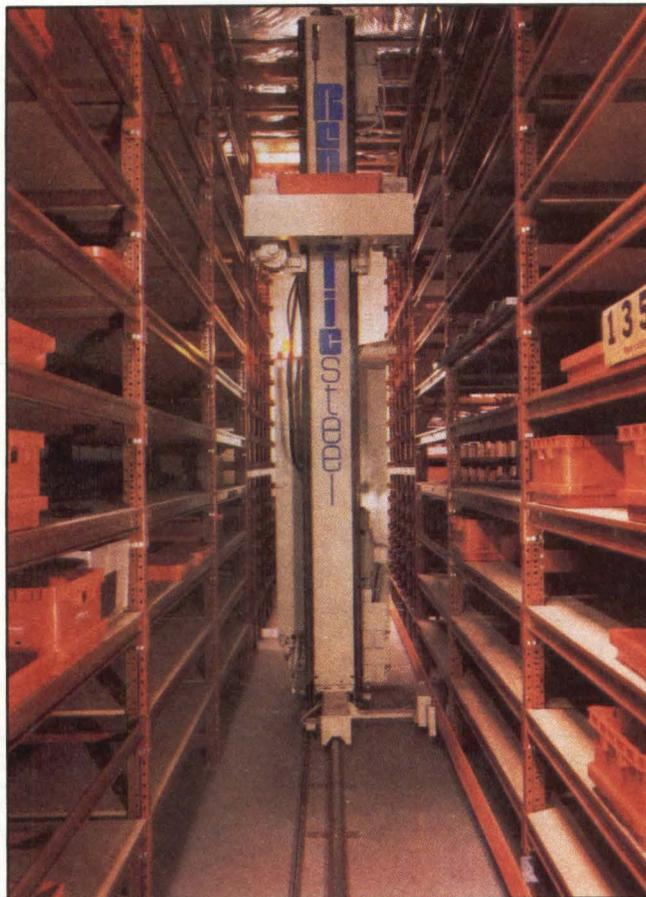
The mini-load AS/RS (like the one shown here) is considered by most suppliers of material-handling systems to be their most standardized piece of equipment. Yet marketing manager Roy Ferrari of Harnischfeger admits that software must be customized even for the mini-load. "I don't think we'll ever reach the point where we can say, 'Here's a standard software package,'" he says.
