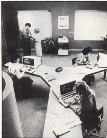
**Honeywell's DPS 6/40 16-bit small-business system supports four to 18 users with as much as 1M byte of main memory (expandable to 2M bytes early next year) and can access more than 1G byte of on-line disk storage. It runs Honeywell's multifunctional MOD 400 operating system for concurrent transaction-processing, office-automation, program-development and data-communications tasks.**
