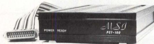
MSI's PCT-100 IS A CONFIGURABLE IN-LINE RS-232 PROTOCOL AND DATA TRANSLATOR WHICH CAN PROVIDE:
