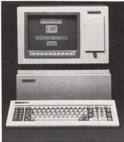
LinkData's packaged system based on the IBM Computer System 9000 is claimed to run on the full range of DEC DIBOL software. List price of a typical two-user system with 256K bytes of main memory and a 10M-byte fixed/removable Winchester disk is \$19,720.
