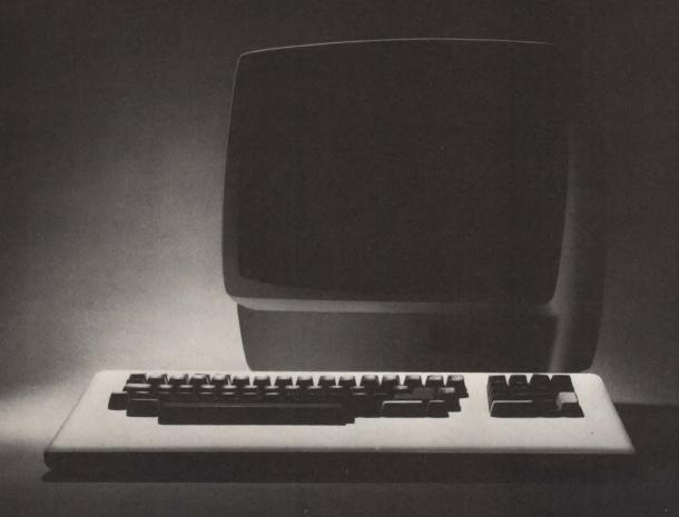
The **Log 200** is Emulog's best user oriented terminal yet. The **Log 200** is completely compatible with the D200 and the DG6053. It comes standard with features like Reverse Video, Detached Keyboard, Sculptured Keycaps and Adjustable Monitor Tilt.
