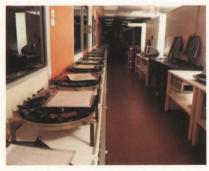
In the main clean room section, the actual assembly takes place on six clean benches. Each engulfed in its own additional bubble of even cleaner air.
