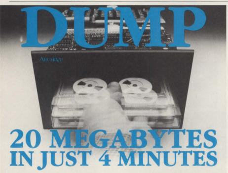
THAT'S PERFORMANCE! That's the Archive **Sidewinder.** It packs more formatted data—up to 20 Mbytes on a single 450 ft. ¼-inch cartridge—more than any other type of Winchester backup storage system. And with 97% tape efficiency.
