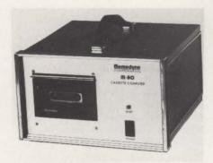
DATA-COLLECTION COMPUTER. The M80 data-collection computer, designed to operate in environments too severe for disk drives, printers and other peripherals, is a self-contained system with a rugged carrying case and its own power supply. Based on a z80 microprocessor, the unit includes a patented high-speed cassette drive capable of handling continuous data streams at rates as high as 9600 baud. Modem and terminal RS232C and TTY current-loop ports are also included. A 2K PROM can be programmed to
