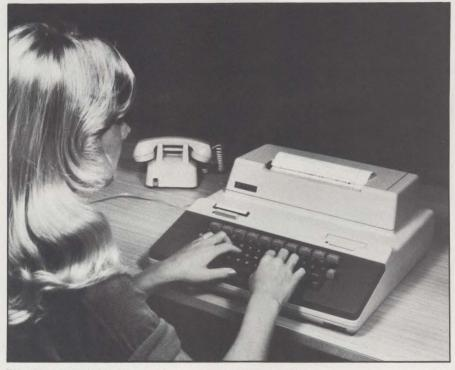
The Hewlett-Packard 2675A portable printing terminal includes built-in modem and thermal printer.
