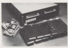
CARTRIDGE TAPE CONTROLLER. The IC-180, a full DMA cartridge tape controller for the DEC PDP-11, emulates the TM-11/TU-10 ½-in. magnetic-tape system. Built-in trimode formatting enables users to select drive type and format with densities from 1600 to 6400 bpi. The controller mounts in any two adjacent SPC slots and connects with the cartridge drive via two ribbon cables. Western Peripherals, Tustin, Calif. Circle No 249
