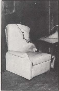
After adjusting all test instruments hanging from the ceiling, left, fire inspector Vern Begley gets set to start a fire in the Los Angeles test facility. In center photo, flames have spread from wastebasket to furniture in about three minutes. Damage from the fire, right, was kept to a minimum by test sprinkler system.
