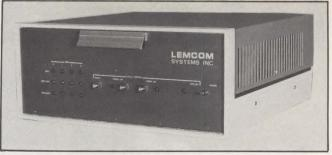
The Lemcom Systems CMC-4 is based on an 8-bit microprocessor.
