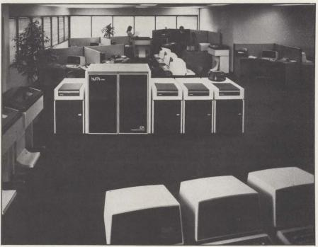
Computer Automation's System 2000 is aimed at large-scale distributed data-processing environments that are typically hosted by an IBM mainframe.
