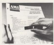
DATA-LINK CONTROLLER. The s6854 data link controller, designed for s6800 and other 8-bit parallel-bus microprocessors, performs communication-link functions for the advanced data-communication control procedure (ADCCP), high-level data-link control (HDLC) and synchronous data-link control (SDLC) standards. The s6854 provides the data-communications interface for primary and secondary transmitting stations in
