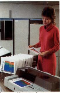
A new graphics plotter from Hewlett-Packard, with eight color pens and automatic cut-sheet paper feed, produces 11-by-17-inch hard copies.
